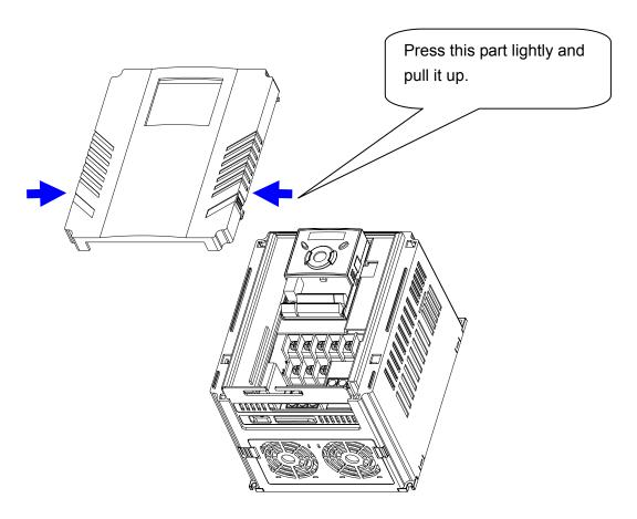
To change the inverter fan: Press the both sides of bottom cover lightly and pull out to your side.
