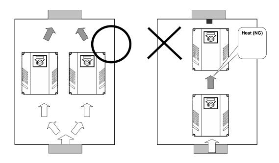
Note: Take caution on proper heat ventilation when installing inverters and fans in a panel.
